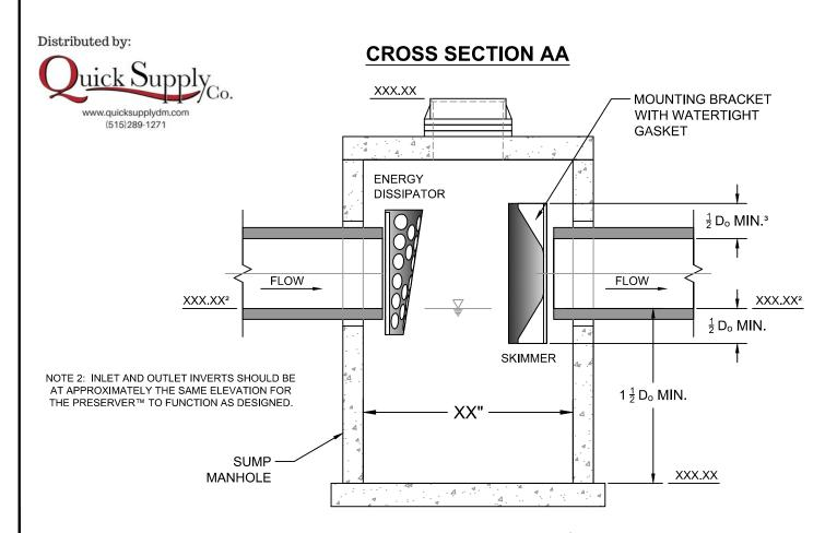
NOTE 3: STOCK SKIMMERS HAVE A FREEBOARD DEPTH OF  $\frac{1}{2}$  D<sub>0</sub>. FOR GREATER FREEBOARD DEPTHS, DESIGNERS CAN UPSIZE THE SKIMMER, OR USE A CUSTOMIZED SKIMMER. FOR CUSTOM DESIGNS, AND/OR PROJECT SPECIFIC DETAILS, CONTACT MOMENTUM.
